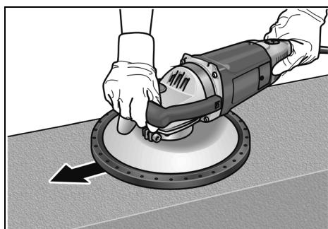
7. Increase the pressure to bring the sanding pad into contact with the work surface. In doing so, slew the renovation sander with overlapping movements.
