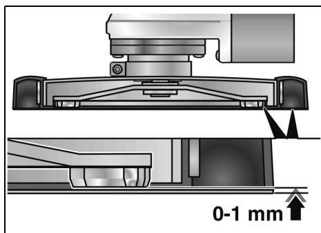
The rubber extraction ring should protrude over the sanding pad by approx. 0–1 mm. If required, correct (see "Adjusting the guard").
